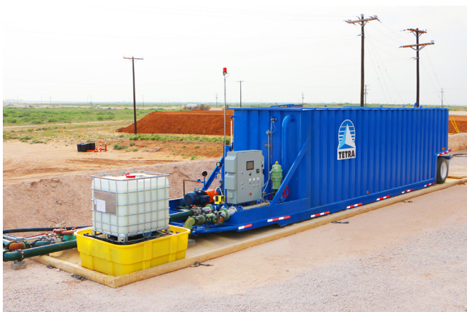
Figure 3. ORapt water/oil separation unit.
