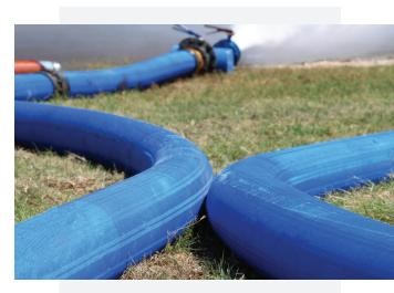
An operator sought a more efficient and reliable means of water transfer at an expansive pad site located on a cattle and horse ranch. TETRA automated the water management and installed 13 miles of TETRA Steel lay-flat hose that ultimately transferred 50,000 barrels of water per day.
